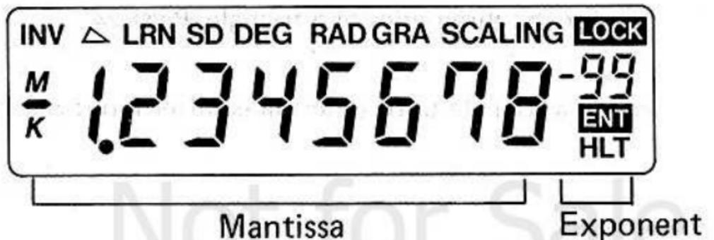
The Display shows input data, interim results and answers to calculations. The mantissa section displays up to 8 digits. The exponent section displays up to  $\pm 99$ .
