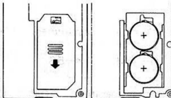
4. Take out the old batteries and replace with new batteries. Be sure the positive (+) sides face up.
